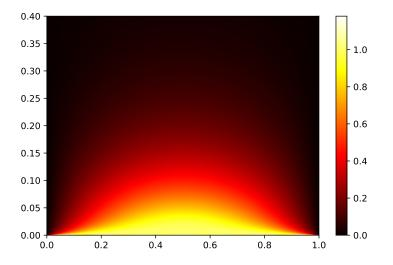
Can you make sense of the plot? Does that plot confirm our expectations? [Note that the horizontal axis shows x for  $x \in (0, 1)$ , while the vertical axis shows t for  $t \in (0, 0.4)$ . Yellow represents 1 (for t = 0, all values are 1 because of the initial condition), while black represents 0.] The boundary conditions in the next example model insulated ends.
