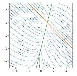
Because both eigenvalues  $\begin{pmatrix} -1 & \text{and} & -6 \end{pmatrix}$  are negative,  $\begin{bmatrix} 1 \\ 2 \end{bmatrix}$  is an asymptotically stable equilibrium point. More precisely, it is what is called a **nodal source**.
