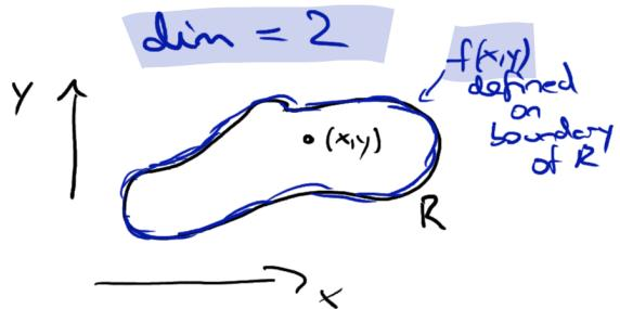
$$\left. \begin{array}{l} u_{xx} + u_{yy} = 0 \quad \text{within region } R \\ u(x_1, y_1) = f(x_1, y_1) \quad \text{on boundary of } R \end{array} \right\} \text{Dirichlet problem}$$
