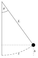
**Solution.** (Newton's second law) The tangential component of the gravitational force is  $F = -\sin\theta \cdot mq$ . Combining this with Newton's second law, according to which  $F = ma = mL\theta''$  (note that a = s'' where  $s = L\theta$ ), we obtain the claimed DE.
